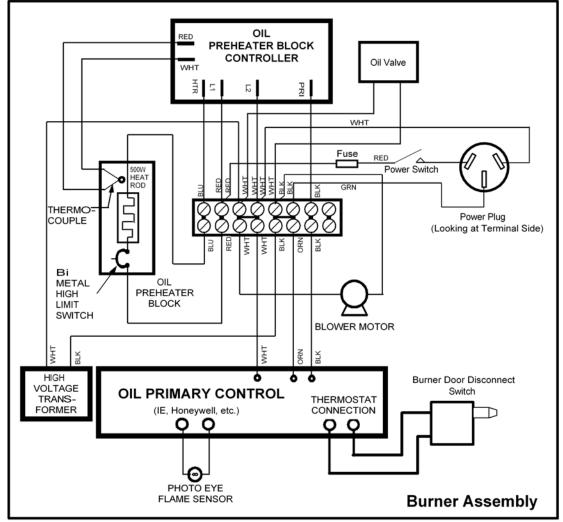
Figure 34. WIRING DIAGRAM, SINGLE HEATING ZONE ONLY (BOILERS EQUIPPED WITH BURNER DOOR DISCONNECT SWITCH)
